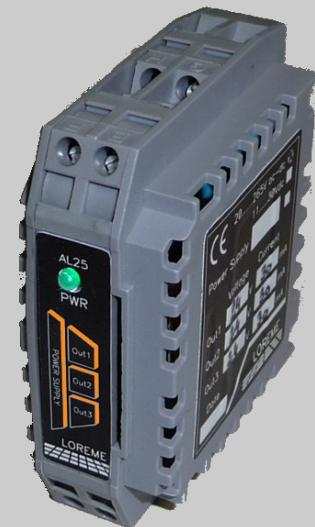
The standard version of the AL25 is intended for separated power of 4 ... 20mA current loops. Very compact and fully protected, it is available in 1-3 isolated outputs, current limited to protect the sensor in case of a default on the loop. This power supply can be declined for any output voltage, single or symmetrical.
